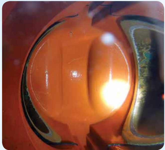
An under-pressure look of clean valve seat.
