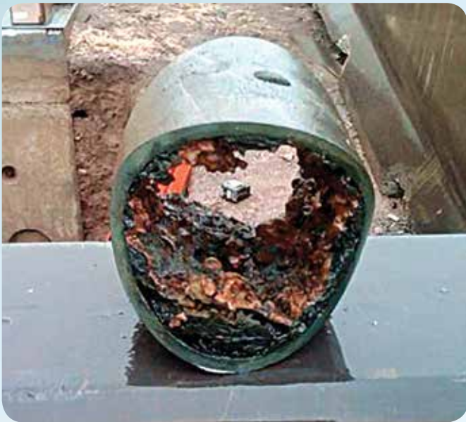
Typical pipe with internal obstructions. InsertValve gate sits on the valve body and not the host pipe.
